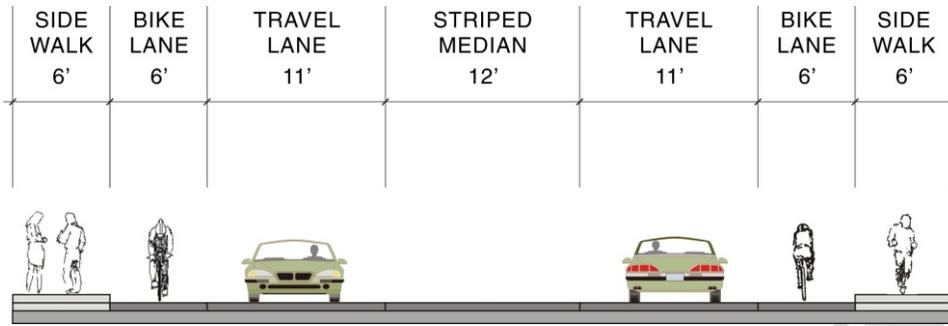
Variations of the basic cross-section above can be explored in locations with more existing paved right-of-way. Traffic operations analysis was performed for the Maple Street/North Main Street (OR 99) and Wimer Street-Hersey Street/North Main Street (OR 99) intersections. The lane configurations at those two intersections would be modified to fit the proposed road diet cross-section. The modified lane configurations and findings from the traffic operations analysis are summarized in Table 2.
